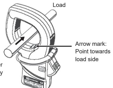
Reverse clamping switches the symbols (+/-) for active power (P).
