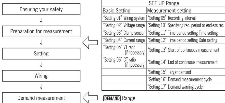
\* Measured demand values will be displayed on the LCD at the start of measurement.
