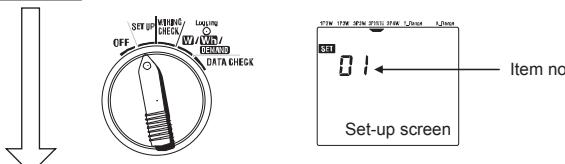
**STEP2** Use the Cursor keys and switch the Setting items with Setting no. 01 to 27.
