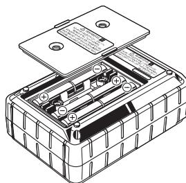
Install batteries in correct polarity as marked inside.
